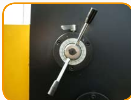
Comando variazione interspazio lame a volantino centralizzato Control of the gap between the blades by means of a centralized hand wheel
