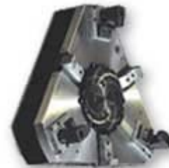
automatic chuck for alloy wheels clamping centering by means of 3 radial jaws clamping by means of 3 axial arms
